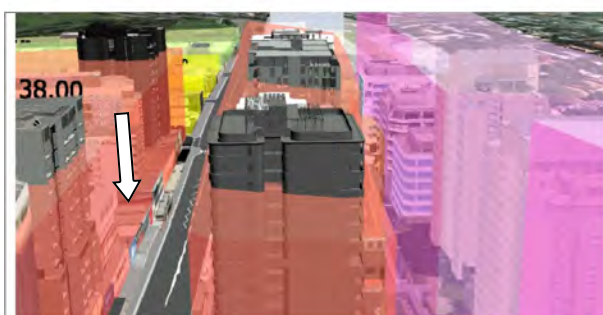
Figure 16: Snapshot from the Waverley Digital Model, looking west above Newland Street road reserve and showing three dimension planes of height of buildings development standards applying to the site and its surrounds overlaid by models of existing, recently constructed and approved development (subject development in the centre of snapshot)
